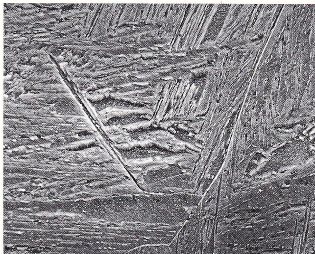
Fig. 6 - SEM of structure of melted zone as welded (2500 x).
