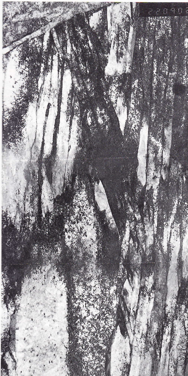
Fig. 7 - TEM of structure of melted zone as welded (33,000 x).
