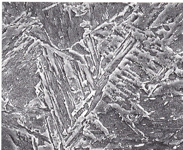
Fig. 8 - SEM of structure of laser-annealed melted zone (2500 x).
