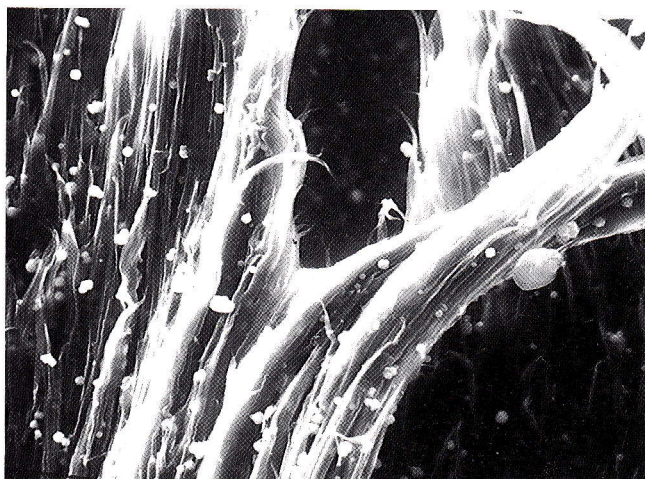
Fig. 15 - SEM photograph at 500 magnifications of a sample jointed by polyethylene holding 10% of filler.
