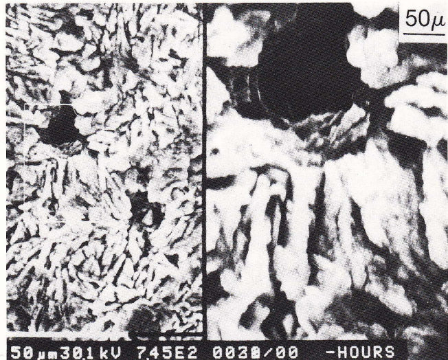
Fig. 12 - (SEM) analysis of the matrix after extraction of ferrite and martensite particles.
