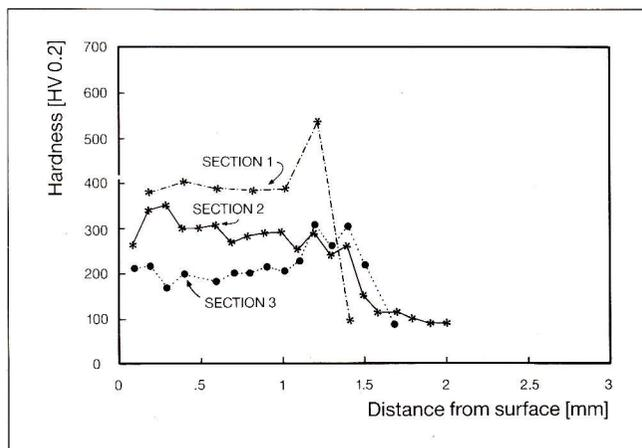
Fig. 5 confirms the one-to-one correspondence between hardness and composition of the layer, as defined by (3). Note that the composition values given in the graph were obtained from micro-analyses made inside the hardness test impressions.
