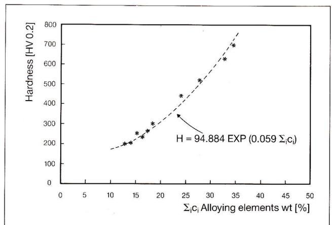
is the best fit of the experimental points, referred to the various process parameters considered (variation of treatment speed, amount of powder and diameter of the laser spot).
