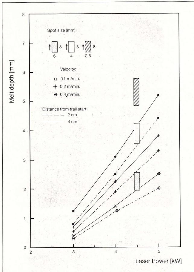
Fig. 1 - Laser surface remelting. Melt depth with regard to process parameters.
