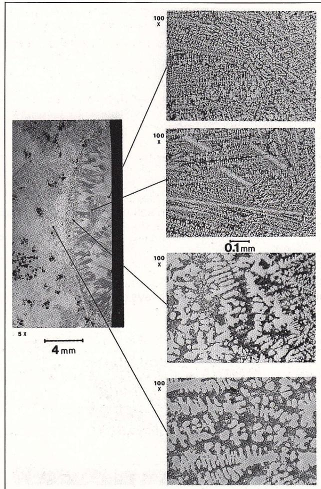
Fig. 2 - Laser surface remelting. Optical micrographs.
