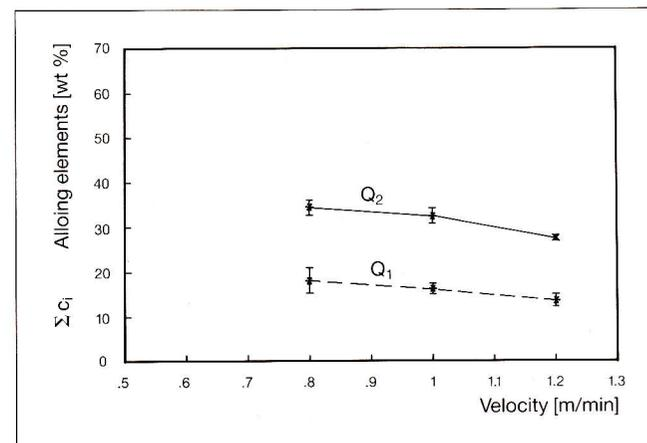
or a partial resolubilization, but rather to a greater dilution of the alloying elements due to the gradual increase in the melted volume during the course of the treatment. This phenomenon is obviously emphasized in the case of specimens with limited mass (as in Fig. 6) while, with larger specimens, there is no great difference between the mean hardness of the individual sections.
