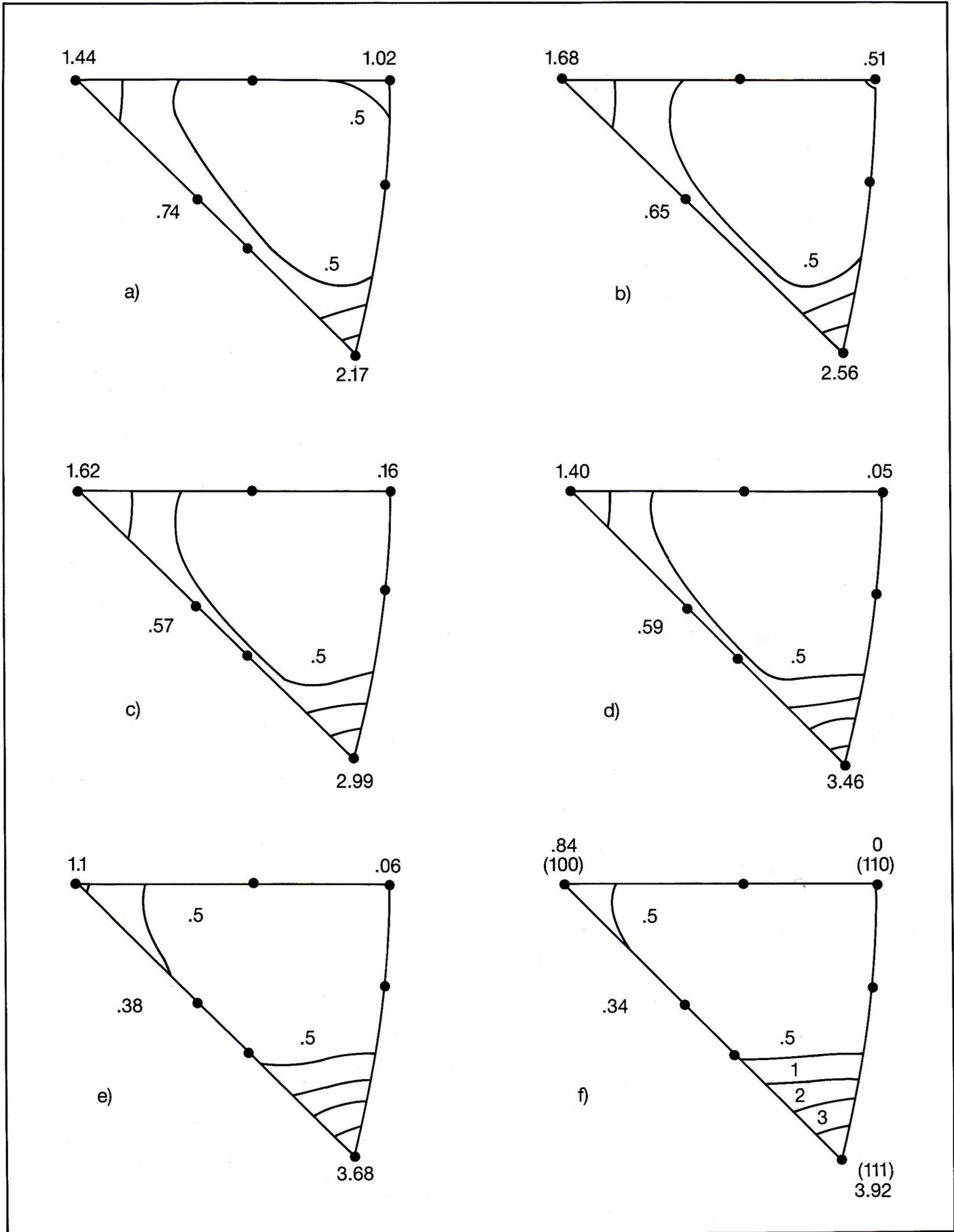
Fig. 2 - Inverse pole figure data showing the density of planes (111) and (100) perpendicular to the rod axis after various drawing reductions.
