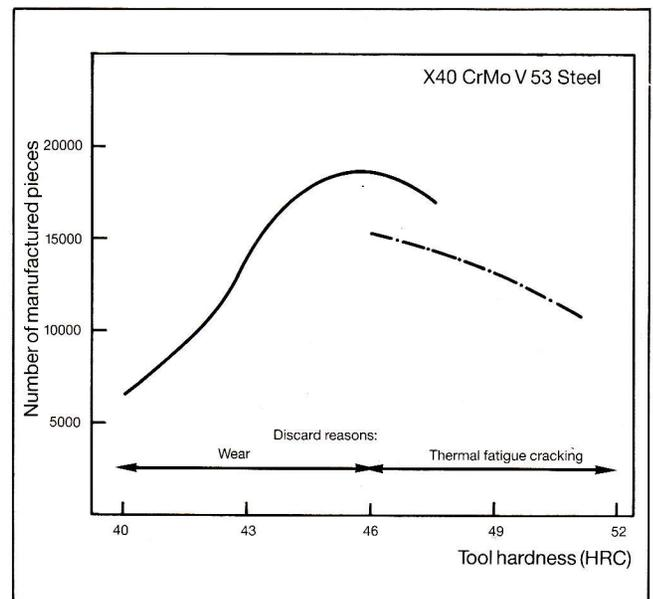
fatigue cracking, tool hardness being, apparently, one of the more influential parameters.
