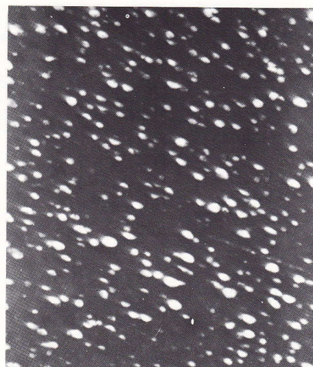
b) \gamma' and \gamma'' phases precipitation (4h);
