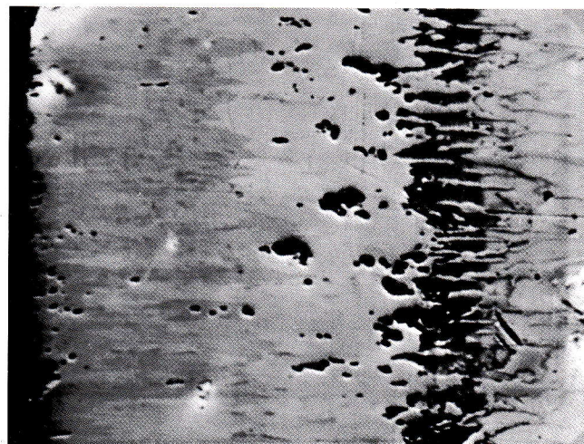
Fig. 1 - SEM micrograph of the borided layer obtained on UNI UX 100 Cr 13 steel ( \times 500 ).
