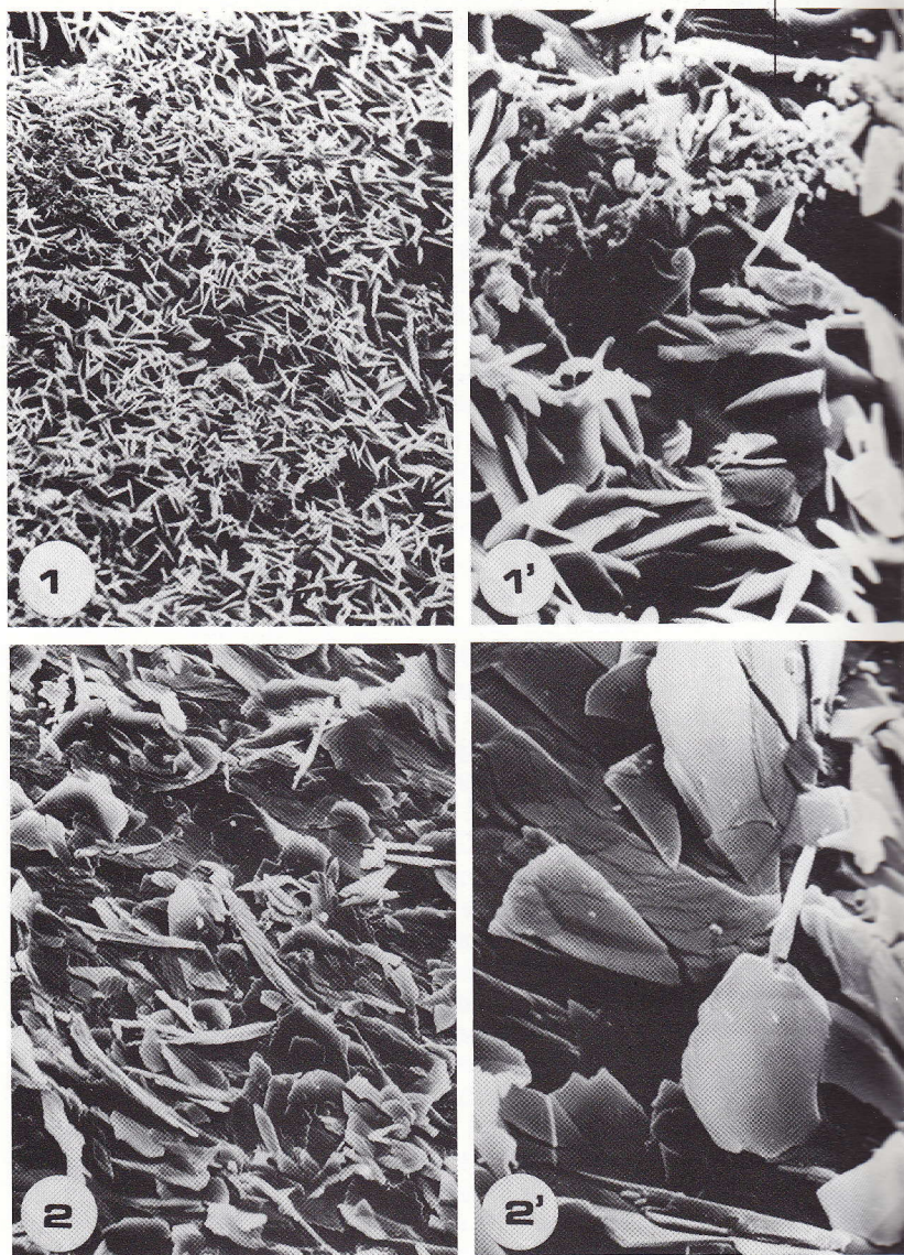
Fig. 1 - SEM micrographies of specimens 1 and 2; phosphate coatings with hopeite structure) 1, 2 (500 ×); 1', 2' (2500 ×).
