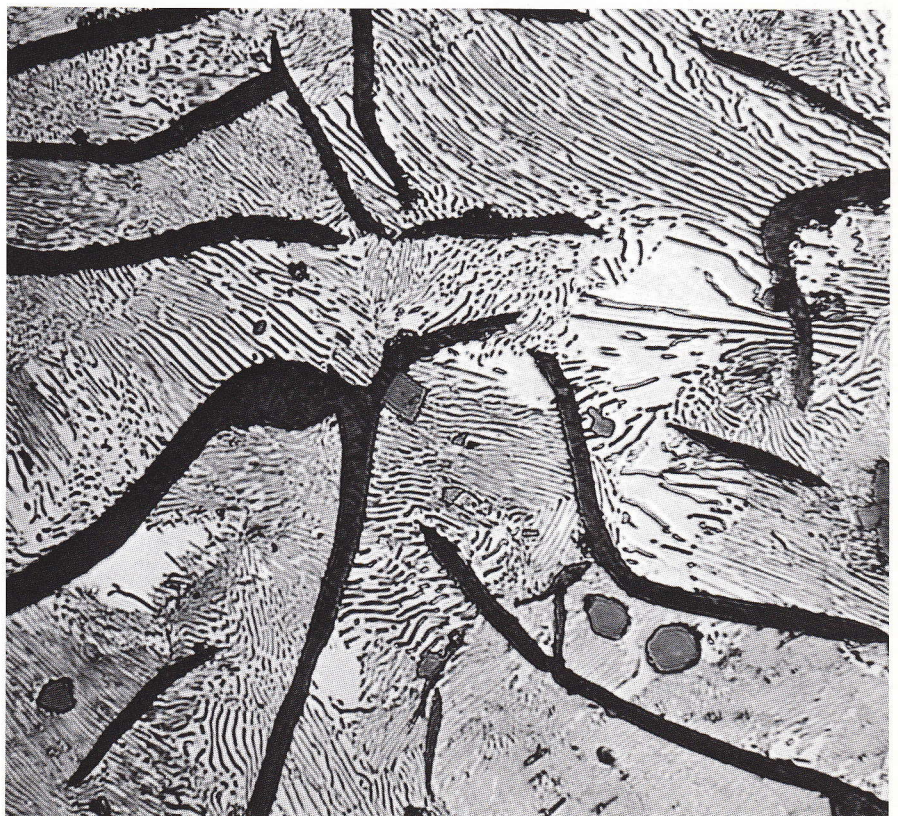
Fig. 8 - Microphoto of flaked graphite grey iron (x 500).
