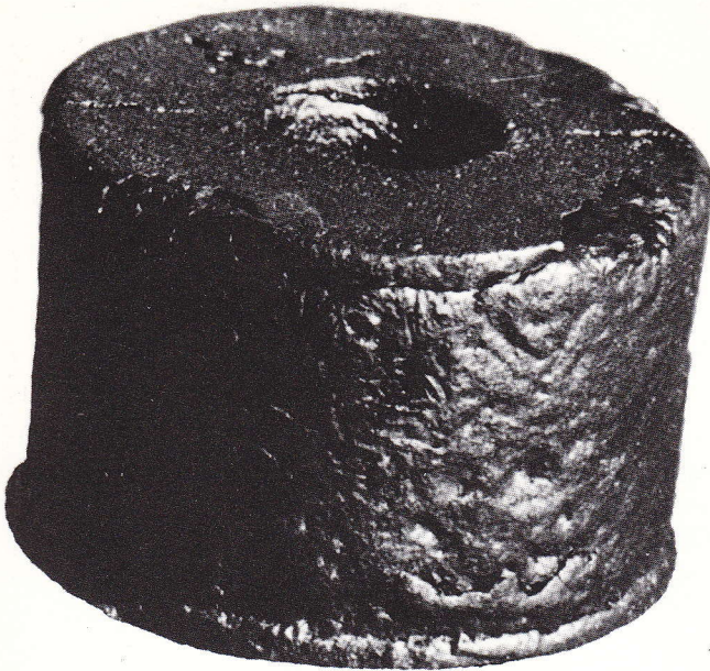
Fig. 10 - Veined appearance of surface due to coat with insufficient gas permeability.
