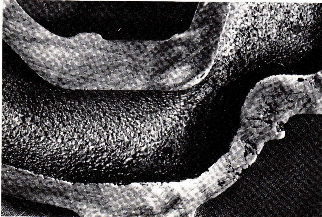
Fig. 9 - Paint penetration into pattern joint face.
