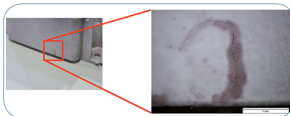
Fig. 4: Lamination revealed by liquid penetrant inspection in sample S6.
