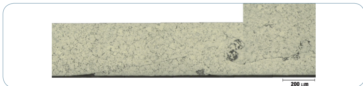
Fig. 10: Presence of continuous bifilm along the surface of Sample S6.
