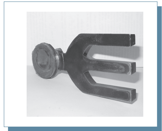
Fig. 1: Fork employed for tensile, fatigue tests and pores volume fraction measurements. Thixocasting was carried out after 30' at 600°C, corresponding to f_s = 0.4 .
