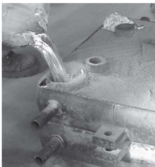
Fig. 2: MMC castings produced according to foundry practice. Pouring of the composite melt in the sand mould (a) and MMC complex-shape casting (b).
