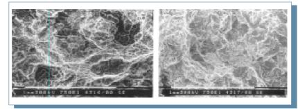
Fig. 5: Comparison of fracture surface before (left) and after LHIP treatment
