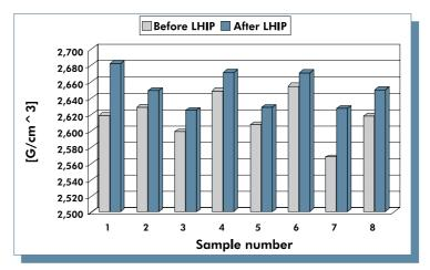
Fig. 4: Comparison of suspension arms density before ad after LHIP treatment
