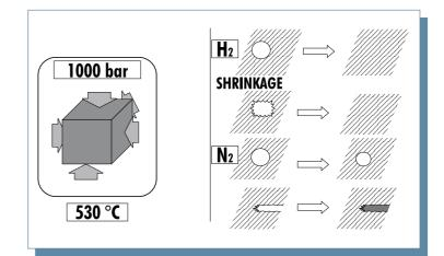
Fig. 3: LHIP process conditions and related effect
