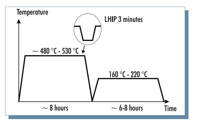
Fig. 6-b: LHIP integration in the H.T. cycle
