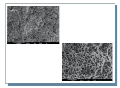
Fig. 7: Fracture morphology of specimens after treatments: 520 °C, 4h+LHIP+ageing 3h at 160 °C
