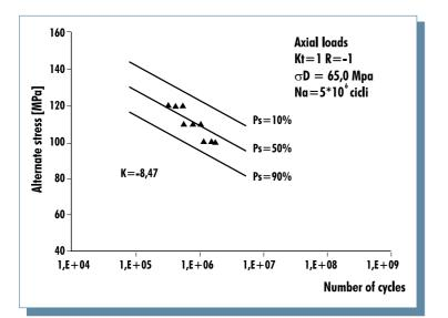
Fig. 8: Wohler curve for the T6+LHIP+T6 trated castings
