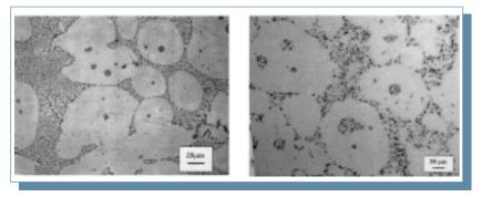
Fig. I: Microstructure characteristics of a feedstock A356 aluminum alloy for thixoforming (left) and of the same alloy after thixoforming
