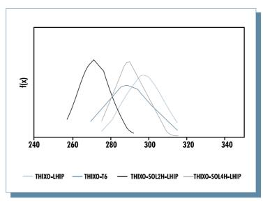
Fig. 6: Gauss distribution of the ultimate tensile strenght
