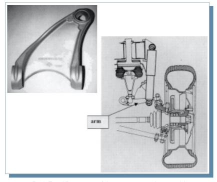
Fig. 4: Two different views of the suspension arm (not in scale)
