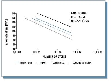
Fig. 9: Comparison between Wohler curves at 50% survival probality of different A356 castings
