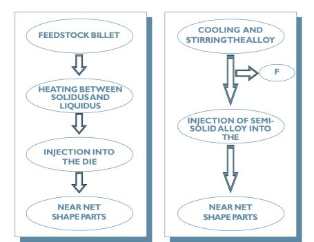
Fig. 2: Process flow steps in Thixoforming
