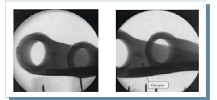
Fig. 5: Radiography of a scrap part, showing the presence of a gas porosity (left picture) before of LHIP treatment and the sound part after the execution of the process
