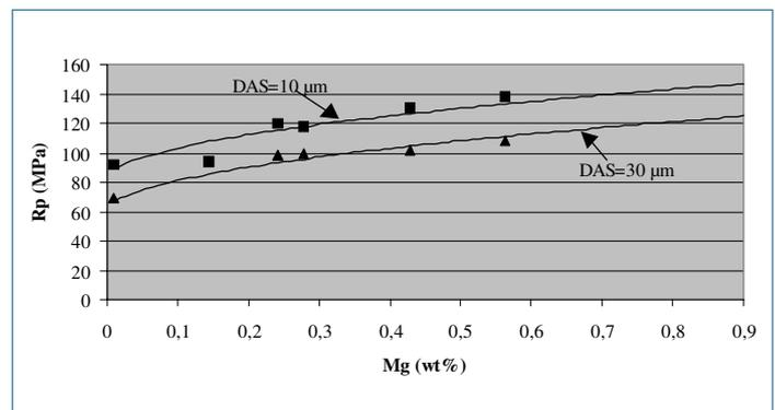
Fig. 1: Calculated as cast yield strength in AlSi7Fe0.1Mg. Squares are experimental results from DC-cast material (DAS = 10  $\mu\text{m}$ ) and triangles from gravity die cast plates (DAS = 30  $\mu\text{m}$ )
