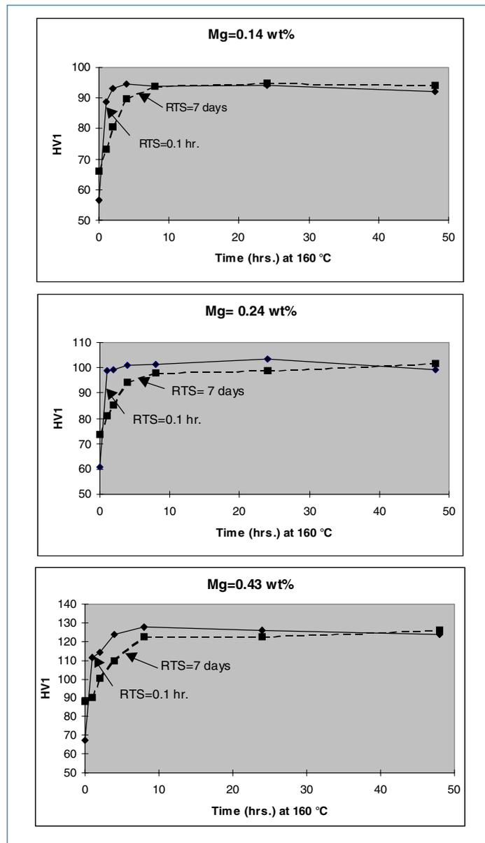
Fig.2: The effect of intermediate Room Temperature Storage time on Vickers hardness after age hardening at 160 °C
