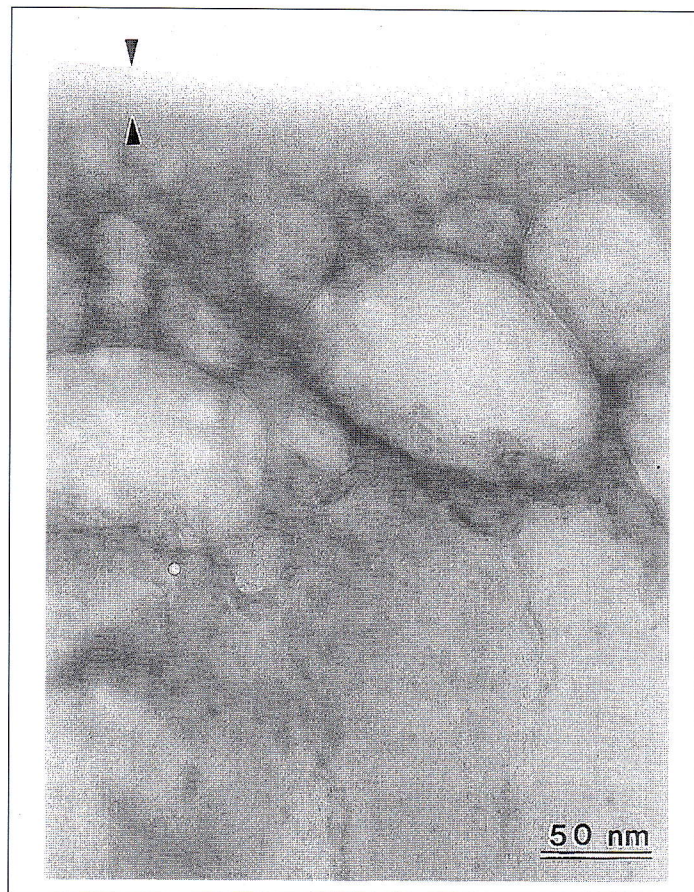
Figure 2: TEM image of an ultramicrotomed cross section of the film formed on pure magnesium after exposure in humid environment, showing a duplex structure with a dense amorphous outer layer (black arrows) and an electron beam sensitive inner layer
