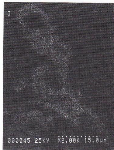
Figure 6c: SEM mapping (X 2000) of the oxygen of the longitudinal section of a formation of chromium oxides for a sample of aluminium coated sintered AISI 316L austenitic steel heat treated at 600°C for 24 h with oven cooling and at 900°C for 24 h with water quenching
