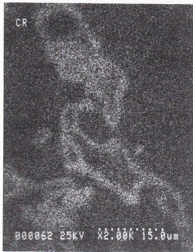
Figure 6b: SEM mapping (X 2000) of the chromium of the longitudinal section of a formation of chromium oxides for a sample of aluminium coated sintered AISI 316L austenitic steel heat treated at 600°C for 24 h with oven cooling and at 900°C for 24 h with water quenching
