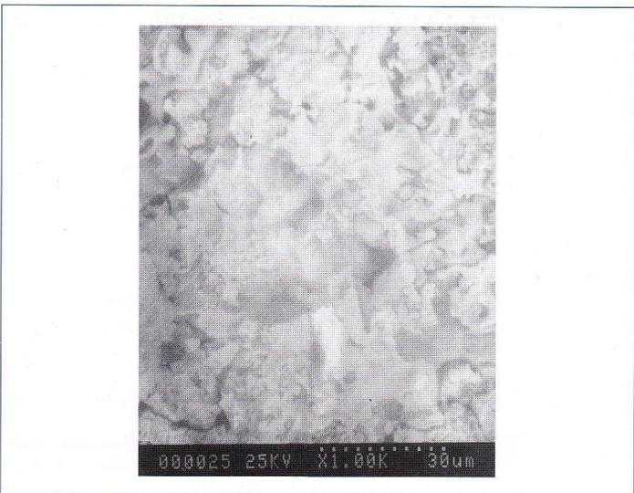
Figure 2a: SEM micrograph (X 1000) of the longitudinal section of a sample of aluminium coated sintered AISI 316L austenitic steel heat treated at 600°C for 24h with oven cooling and at 800°C for 24 h with water quenching. The micrograph refers to the interface of the interdiffusion/matrix area
