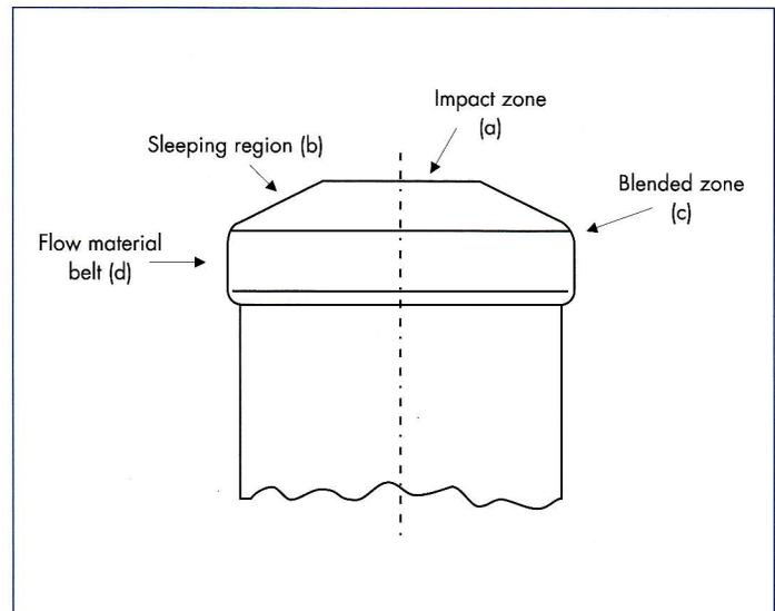
Figure 1: Schematic geometry of an extrusion punch
