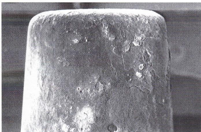
Figure 4: Surface features at the head of the TiAlN core pin in the most critical location after 22000 shots
