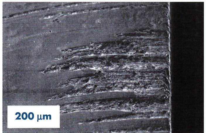
Figure 8: Typical damage on the lateral belt of the TiN coated cool forging tool. SEM micrograph of the surface near the transversal section; longitudinal axis of the punch: horizontal
