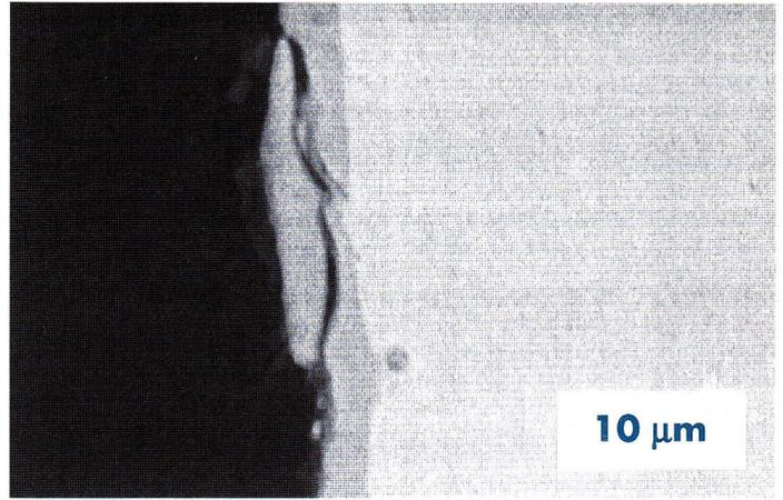
Figure 6: Partial scaling off of the CrC layer in a critical core pin. SEM micrograph of a longitudinal section (the axis of the core pin is vertical)
