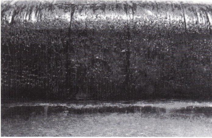
Figure 9: Blended and belt regions of the examined extrusion punch for warm forging after 40000 strokes. The axis of the tool is vertical
