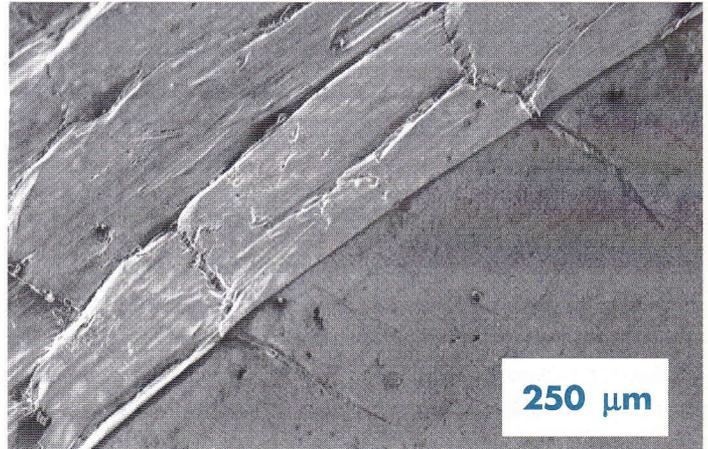
Figure 11: SEM micrograph showing the typical surface and the corresponding longitudinal section (right-bottom and left-upper sides, respectively) in the heavy flow region of the hot forming tool
