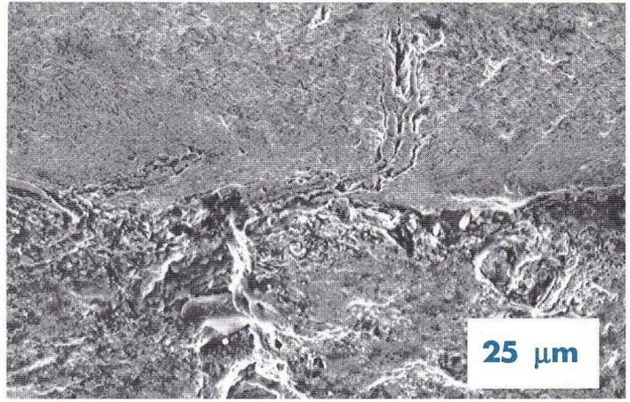
Figure 10: SEM micrograph showing both the lateral surface and longitudinal section (bottom and upper parts, respectively) of the warm forming tool in a region where a circumferentially oriented crack was present
