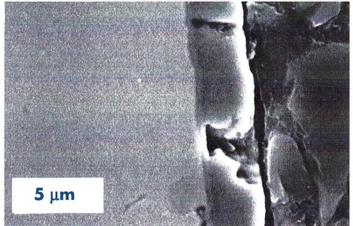
Figure 7: Typical features of an examined TiAlN coated core pin after a service life of 22000 shots. SEM micrograph of a longitudinal section (the axis of the core pin is vertical)
