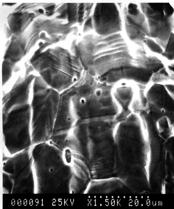
Fig. 9 Intergranular and transgranular attack . (stage 5: -290 mV, 42h, 2,5/0,5) + (stage 4: -150 mV, 30h, 2,5/0,5) x 1500
