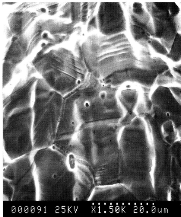
Fig. 8 Intergranular and transgranular attack . (stage 5: -290 mV, 96h, 2,5/0,5) + (stage 2: 780 mV, 46h, 2,5/0,5) x 1500
