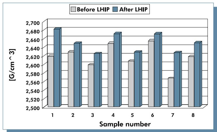
Fig. 4: Comparison of suspension arms density before and after LHIP treatment
