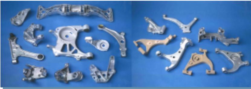
Fig. 1: Solid shape (left) and hollow shape (right) components with cores
