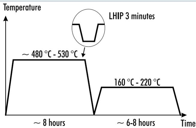
Fig. 6-b: LHIP integration in the H.T. cycle
