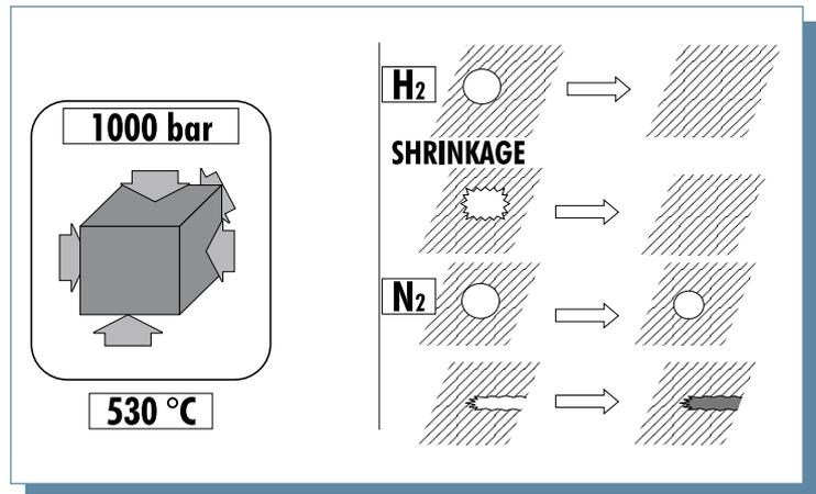
Fig. 3: LHIP process conditions and related effect
