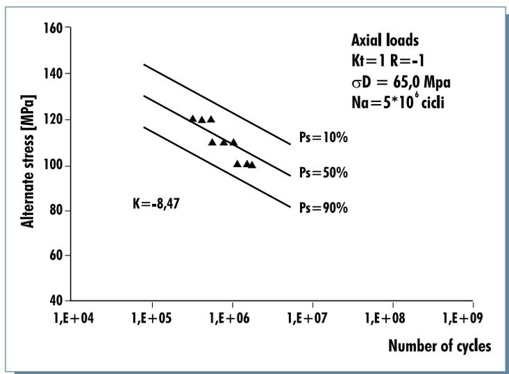
Fig. 8: Wohler curve for the T6+LHIP+T6 treated castings
