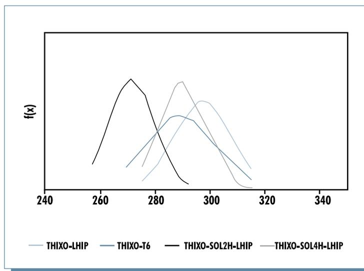
Fig. 6: Gauss distribution of the ultimate tensile strength
