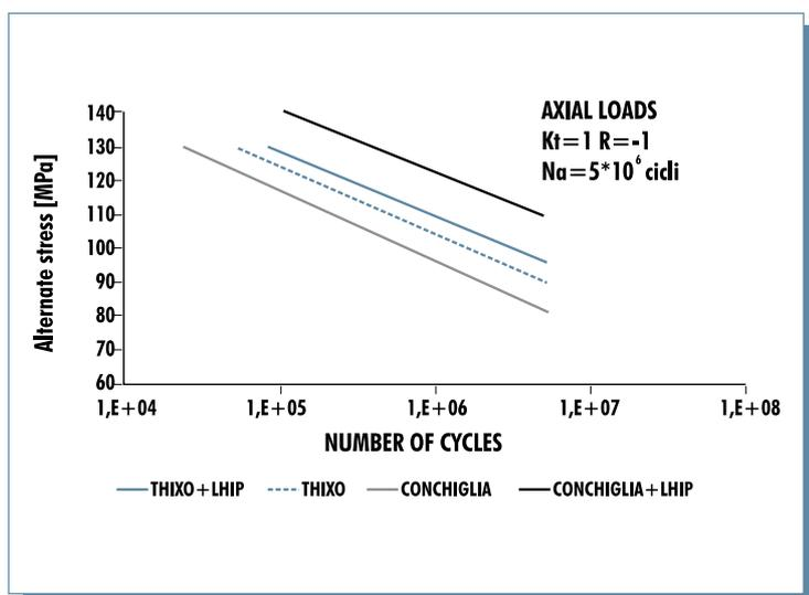
Fig. 9: Comparison between Wohler curves at 50% survival probability of different A356 castings
