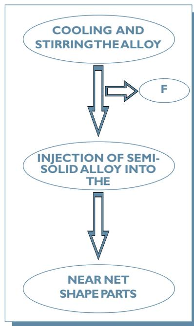
Fig. 3: Process flow steps in Rheocasting, F means feedstock billet for Thixoforming
