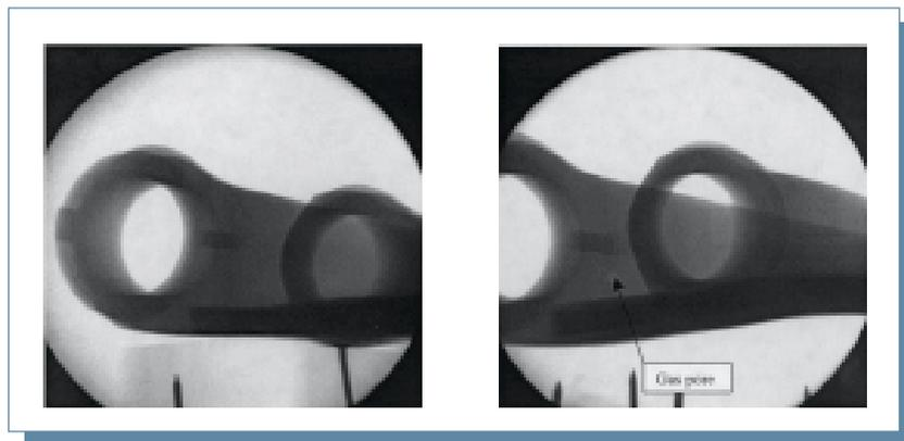
Fig. 5: Radiography of a scrap part, showing the presence of a gas porosity (left picture) before of LHIP treatment and the sound part after the execution of the process
