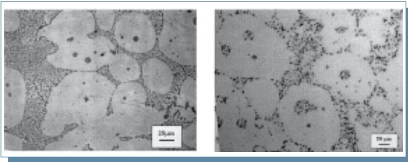
Fig. 1: Microstructure characteristics of a feedstock A356 aluminum alloy for thixoforming (left) and of the same alloy after thixoforming
