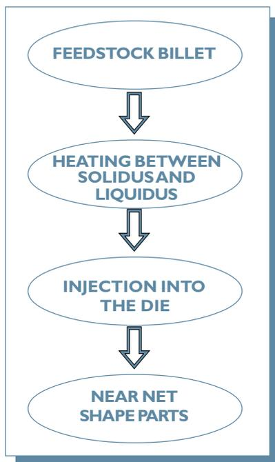
Fig. 2: Process flow steps in Thixoforming
