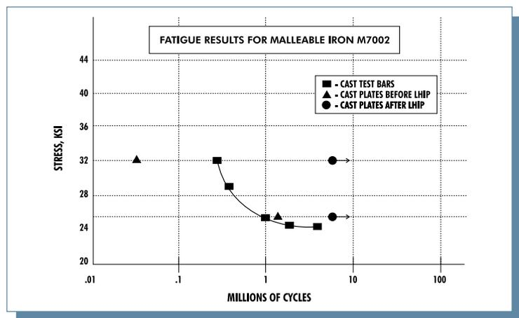
Fig. 3: Some fatigue properties of malleable iron castings
