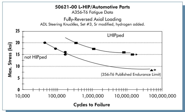
Fig. 2: Some fatigue properties of aluminum castings
